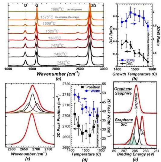
Figure 2: Raman spectroscopy (a-d) of graphene grown on sapphire demonstrating improved structural quality (a,b) with growth temperature, mono and bi-layer graphene (c), and XPS (e) indicating the lack of a buffer layer compared to graphene on SiC.
