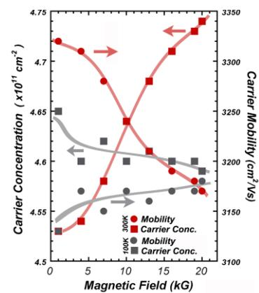
Figure 5: Carrier mobility and concentration of graphene/sapphire grown at 1500°C as a function of magnetic field at 300K and 100K.
