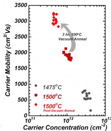
Figure 4: Carrier mobility and concentration of graphene/sapphire as a function of temperature and measurement conditions.
