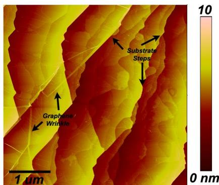
Figure 3: Atomic force micrograph of graphene on sapphire grown at 1500°C. Note the presence of steps in the sapphire substrate and small wrinkles (<1nm high) in the graphene film.
