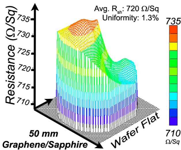
Figure 1: Sheet resistance map of a 50mm wafer of graphene on sapphire demonstrating a high level of uniformity.
